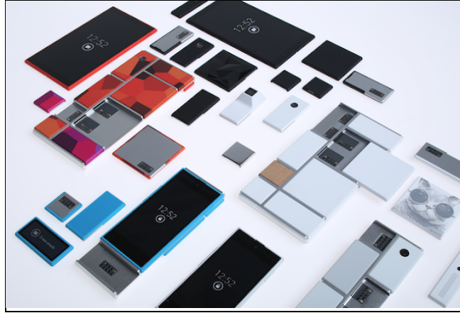
Figure 1-6: Modular smartphones (from the Motorola blog )
